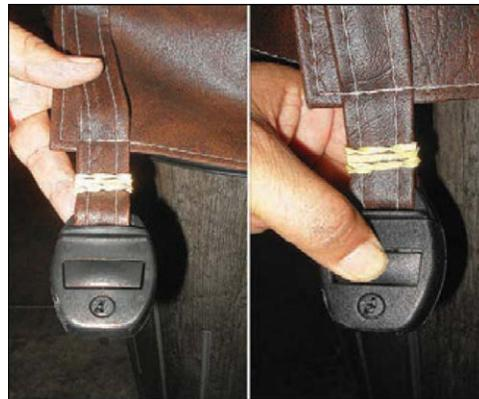
**Step 3** With the straps pulled tight (but not overly tight), lightly pre-drill the location for screw placement. Gently drill 3 holes - one for each screw slot in the lock.
