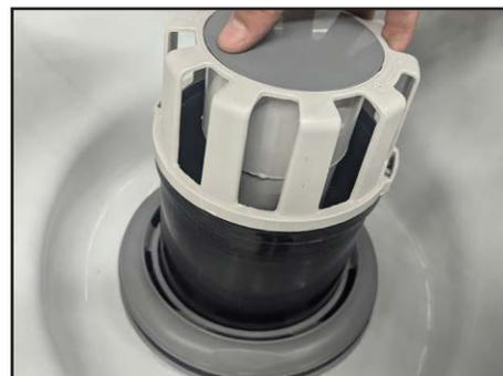
After removing the filter, reinstall the retainer ring to the canister, then reinstall the skimmer, this skimmer must be able to move up and down with your water level. In the following step you will fill your spa with water through the filter canister.
