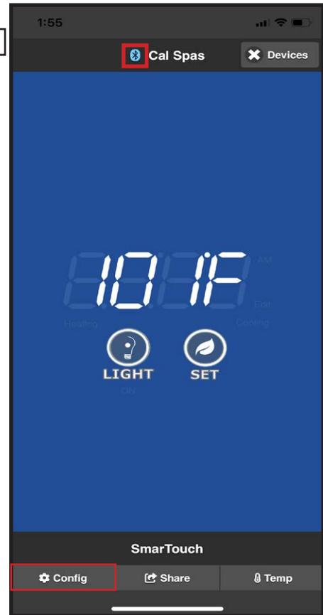
4. The screen will show two buttons for the Light and Set options. The device is currently communicating with your phone via Bluetooth. The next step is to connect it to your local network. To begin select "Config"
